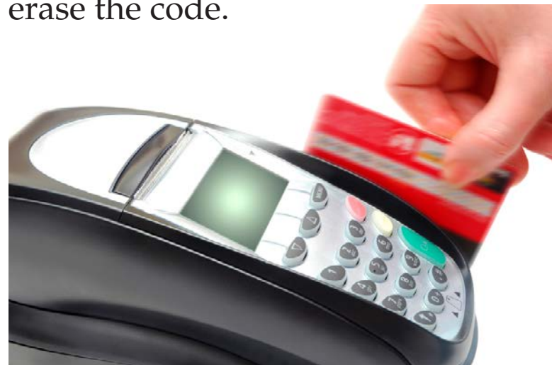
At a store, when someone swipes a credit card, a computer reads that card's code. The code is made of millions of tiny magnets.
