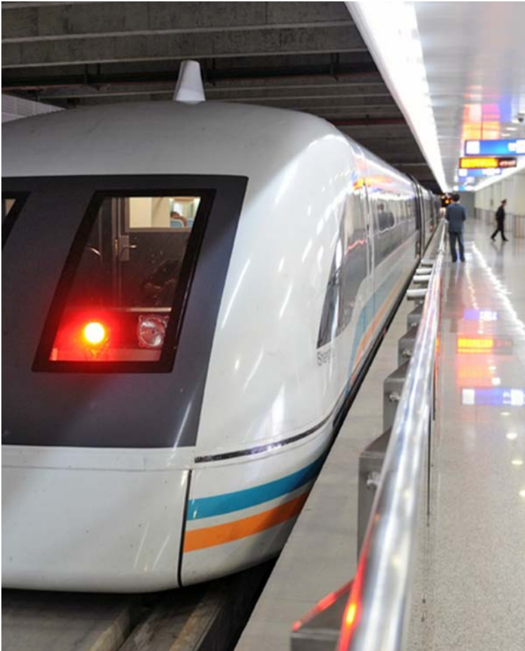
Instead of having wheels like regular trains, this train in China floats on a magnetic cushion between the train and track. It travels at a top speed of about 267 miles (430 km) per hour.
